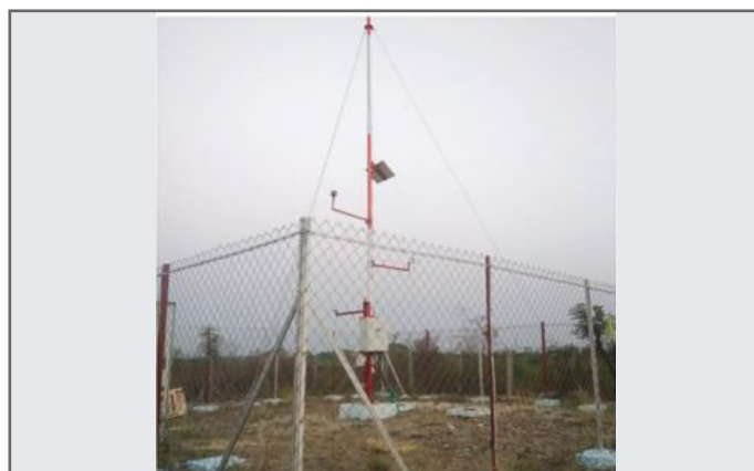
Automatic Weather station
