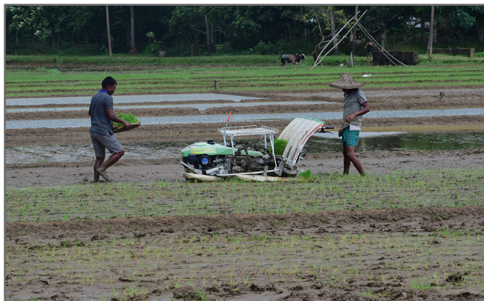
Use of Engine operated walk behind type paddy transplanter
