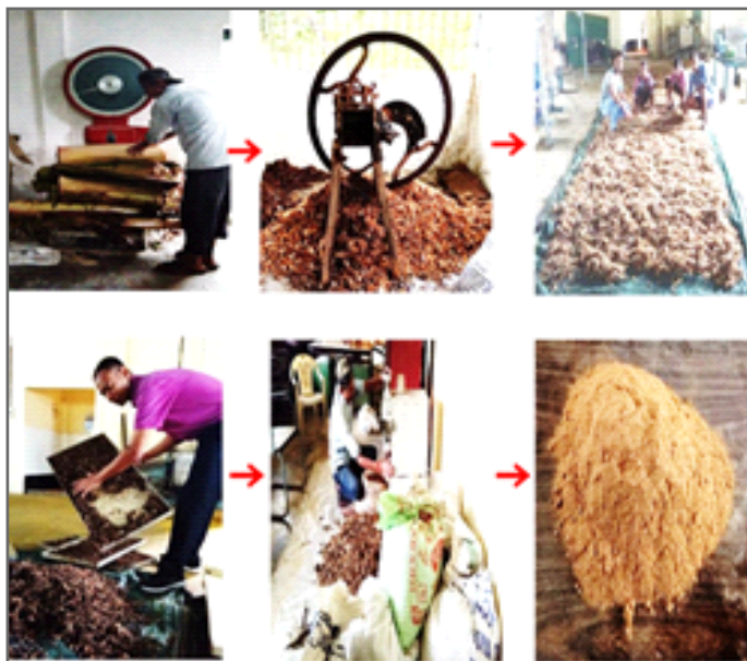
Flowchart of processing of banana pseudo-stem into fine mesh powder form
